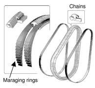
Due to the high friction, the rings require a high fatigue strength, which is obtained by a nitriding process in our production. Currently, we are controlling the nitrogen layer thicknesses by etching in combination with optical microscopy. A micrograph is given in the following picture:
