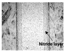
In the near future, we would like to control this nitrogen layer by measurements with our new GDOES equipment.
