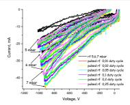
Changing of the current amplitude with the duty cycle can be explained by influence of the discharge power on the temperature of the gas. When the duty cycle increases the mean power consumption increases too, what leads to a heating of the plasma. Under constant pressure according to the thermodynamic law p-nkT an increase of the gas temperature leads to the decrease of Ar atom concentration and therefore of the current.
