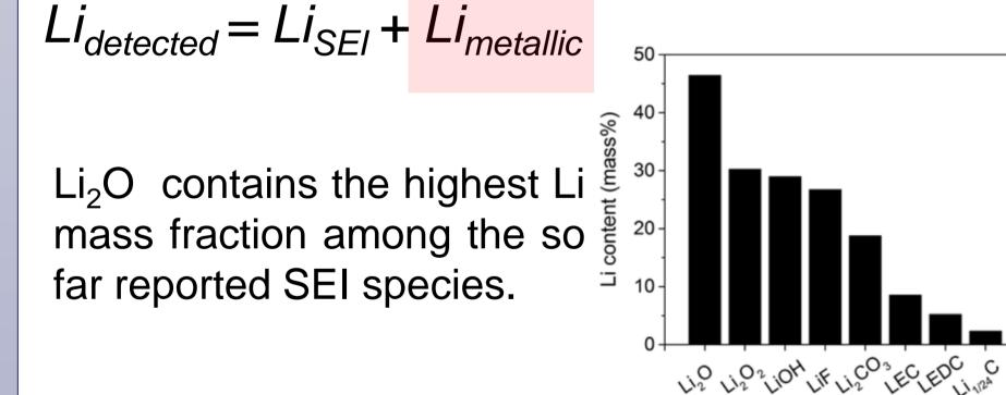
Assuming SEI consists solely of Li<sub>2</sub>O, the SEI contribution in the total detected Li is maximized. Hence, a lower limit is set for the possible amount
