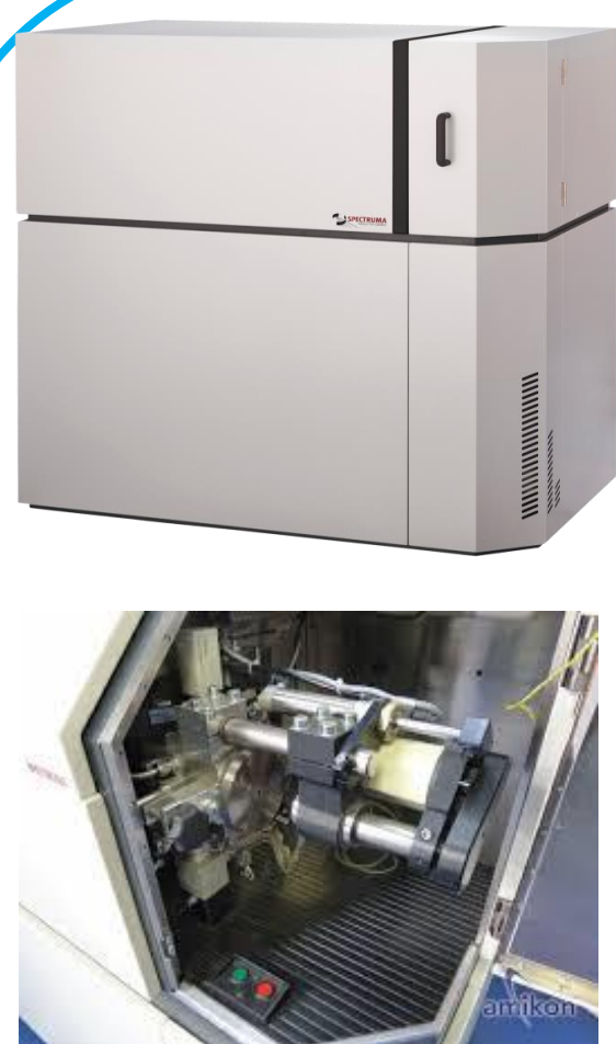
GDA750HR with CCD and PMT detectors (Spectra Analytik GmbH, Hof, Germany)
